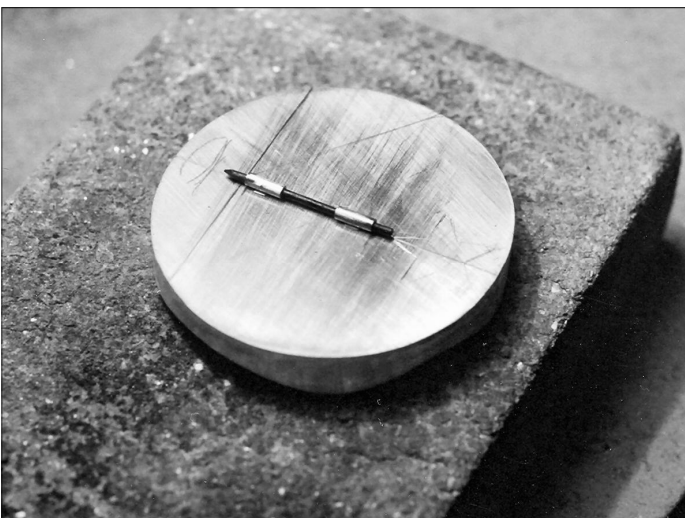
Fig. 5. Hinge on horizontal dial prepared for soldering.
