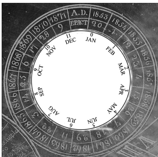
Fig. 5. Suggested index disk for O'Connell's Epact table.
