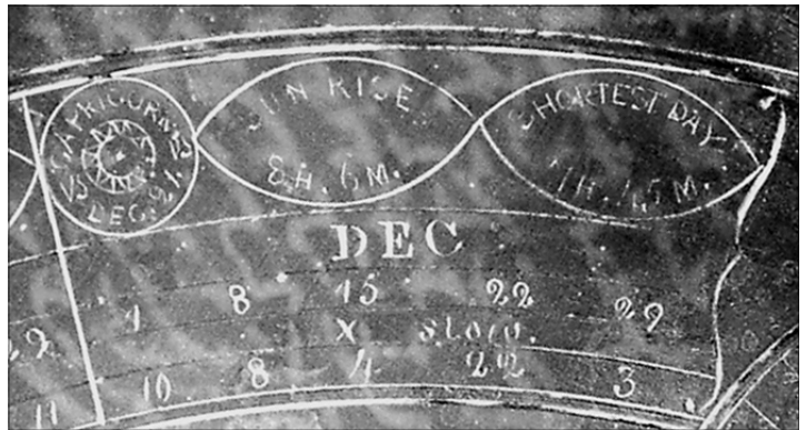
Fig. 7. EoT showing changeover marked with an ‘x’ on 15 th Dec.
