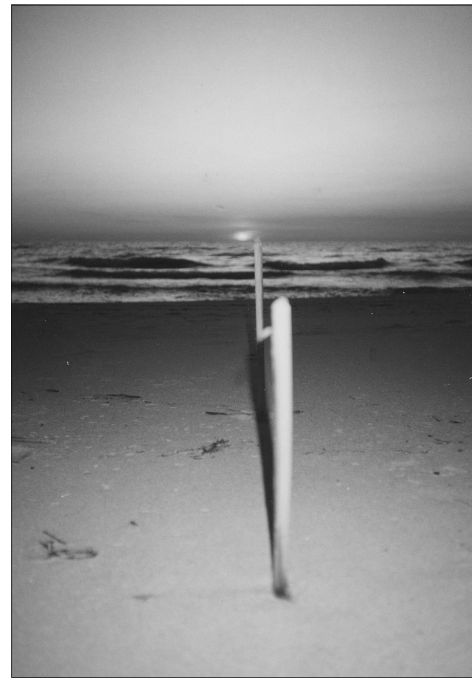
Fig. 5. The two-pole method for marking sunrise and sunset positions on an unobstructed horizon. The Zhou bi ( Chou Pei ) describes the use of this method to determine the meridian halfway between the directions of sunrise and sunset. Pliny the Elder in his Naturalis Historica (II.69) mentioned this method in regard to the determination of the equinoxes. Sunset observation taken 13 May 1993 at Saugatuck by Lake Michigan, Michigan, United States, latitude \phi \approx 42^\circ 40' N .
